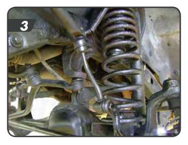
e. Disconnect the track bar from the frame rail bracket. Remove the cotter pin and nut (21mm) and thread it back on a few turns. Strike the track bar frame mount with a hammer to release the tapered seat. Remove the track bar.
