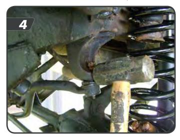
f. With the axle well supported, remove the shocks. Also remove the coil spring retainer located at the rear of the driver side coil mount.
