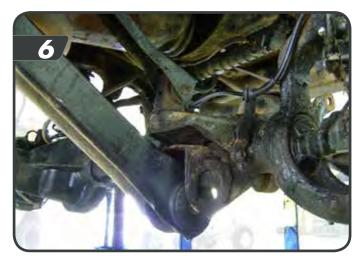
h. Lower the axle enough to remove the factory coil springs. Take care to ensure all hoses have adequate slack and the steering isn't binding. The drag link can be disconnected if necessary.
