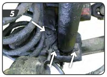
g. Remove the lower control arm to axle bolts.
